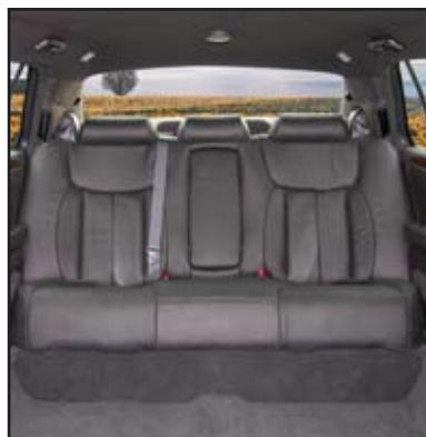
Low profile floor provides the greatest headliner-to-floor clearance. Don't be confused by competitive "flat floor" models that actually raise the floor.
