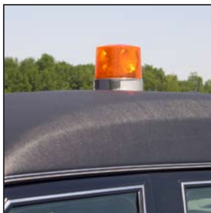
An optional beacon ray light as pictured, or wiring for a customer's light can be installed, if requested.
