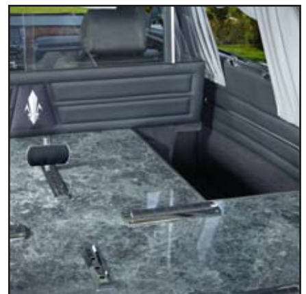
A single front bier pin and open church truck opening are standard on a Statesman.
