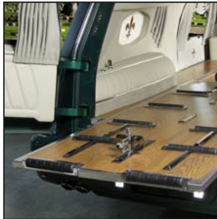
Rear power extend table opens and closes with the push of a button on the rear loading door frame.
