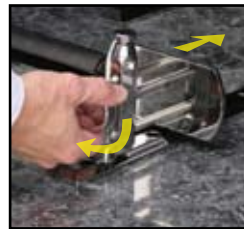
Tighten the quick-adjust knob to secure the casket or Commemorative Carriage in place.
