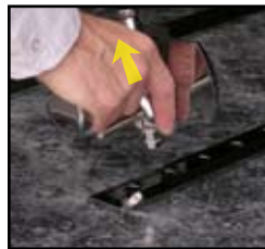
Grasp and pull the Bier Pin straight up from its seated position and...
